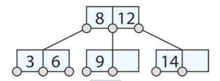
B-trees are "self-balancing," meaning the height of the branches is managed so that they do not get arbitrarily large. Each node contains partitioning "key values" that indicate the values of the children. Their design is optimized for handling very large data files, and for writing data to memory or disk. They are used extensively in database systems like MySQL, PostgreSQL, and Redis, and filesystems such as NTFS, HFS+, and ext4.
