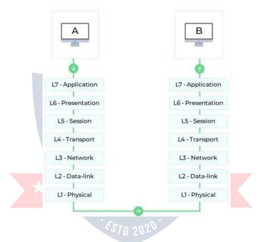
The seven layers in the OSI model can be divided into two groups: upper layers, including layers 7, 6, and 5, and lower layers, including layers 4, 3, 2, and 1. The upper layers deal with application issues, and the lower layers deal with data transport issues.
