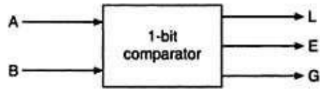
Block diagram of a 1-bit comparator.
