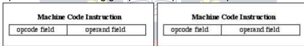
Figure 2: Machine code instruction format
